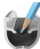
A rubber rim tape presses into the hole of a hollow section rim.
