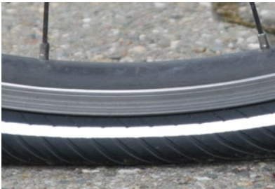
That’s how it shouldn’t look. The inflation pressure is far too low here.
